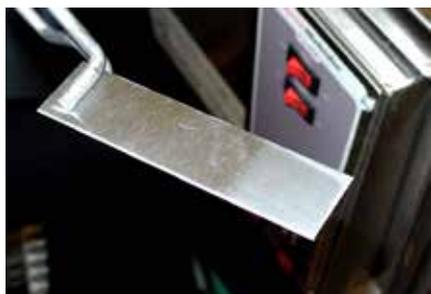
*Illustrating a treated and untreated surface, the thin DuraGlide® coating is visible on the right edge of this steel coupon after partial immersion in the LabKoat system.*
